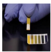
RightSpotpH single-unit packaging prevents pH Paper's exposure to air, light, and humidity. Specimen aspirated into Indicator housing beneath the pH paper.
